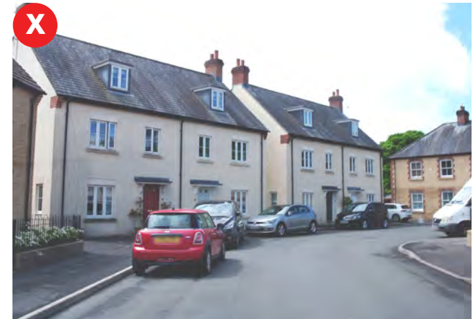
Figure 44: Narrower streets in recent developments with on-street parking can cause traffic pinch points, leading to congestion and difficulty for larger service vehicles to access - these must be avoided and better designed in future developments.
