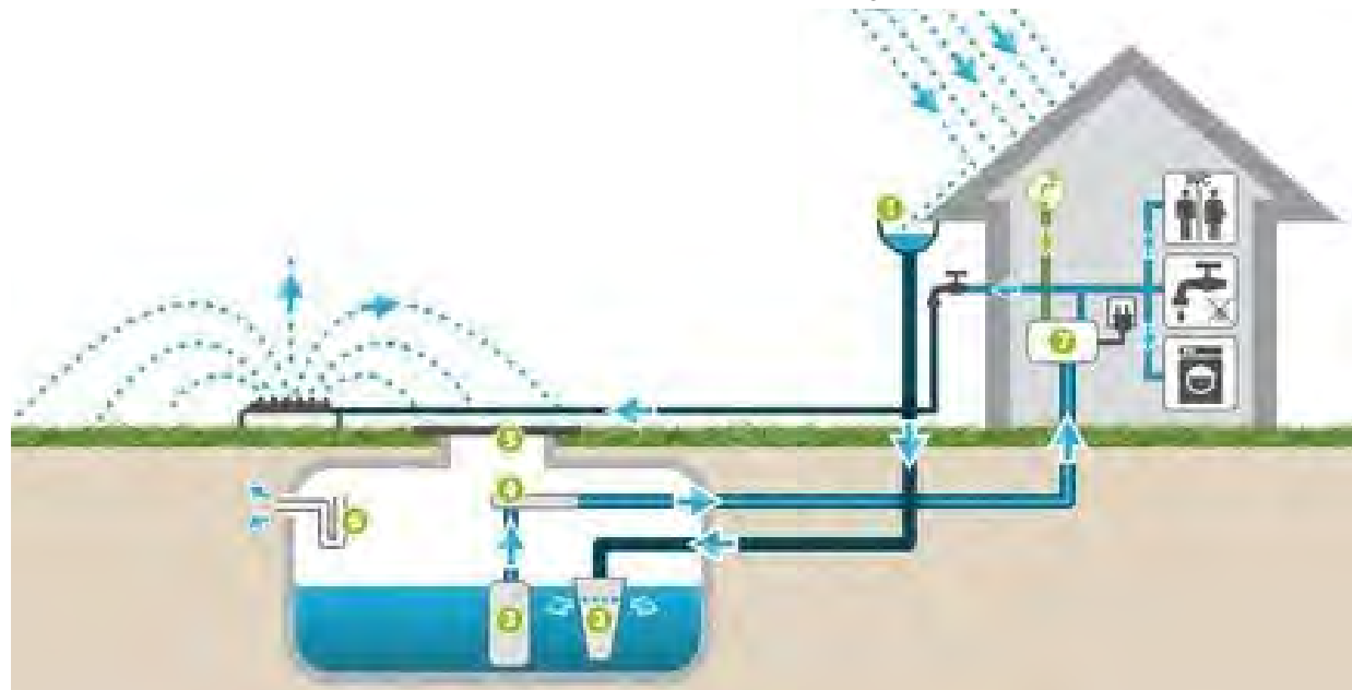
Figure 139: Diagram illustrating rainwater harvesting systems that could be integrated into open space and residential developments.
