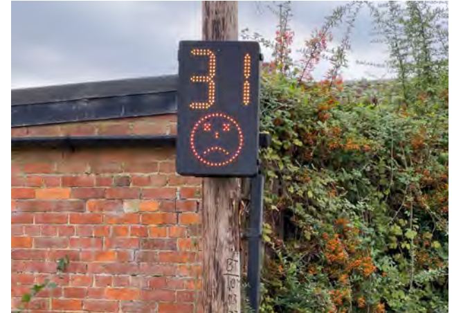
Figure 99: Example of an interactive signage to indicate speed limits within a residential area, Stockley.
